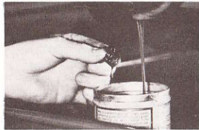
Drain and flush apron every 3 months.
