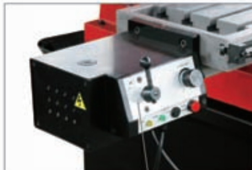
S/N 10141 Power feeder
