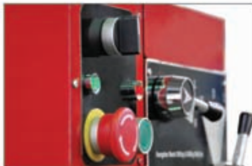
6 steps speed control For/Rev switch & Emergency stop
