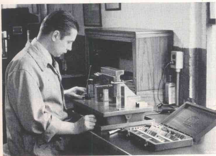
Fig. 4. Checking a Fixture with Precision Surface Plate and Lapped Gauge Blocks
