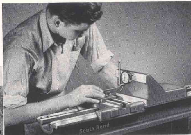
Fig. 7. Above—Testing the Saddle Cross Slide Dovetail for Squareness with V-Ways of the Lathe Bed
