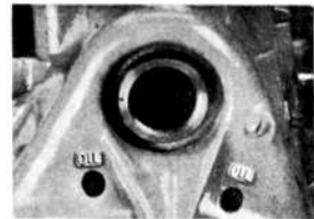
Oiling Points for 10" & 16" Lathe twin gears
