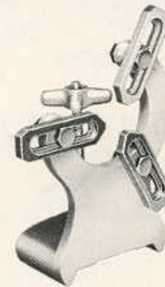
229 Fixed steady with 3 jaws, maximum opening 2"
