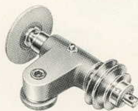
235 Grinding attachment running in adjustable precision taper roller bearings, can be regulated in height, with drawbar for B 8 collets, maximum spindle speed 20 000 r.p.m.
