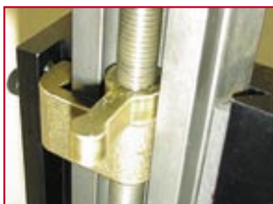
Figure 18—The saddle locking lever provides a positive lock for the Z-axis and is standard on all Sherline manual mills. CNC mills have a lock that also controls backlash.
