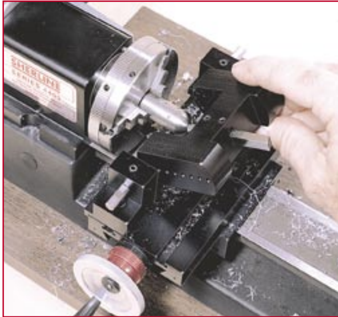
Figure 13—The radius cutting attachment can cut a convex or concave radius. Unlike most lathe operations, the tool is moved up and down rather than horizontally.
