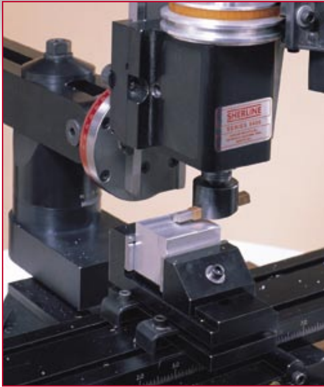
Figure 33—Fly cutting is an excellent way of producing a flat surface quickly. This Model 5400 mill has been converted to 8-direction capacity with a P/N 5650 column upgrade. The adapter base can be seen in the background.
