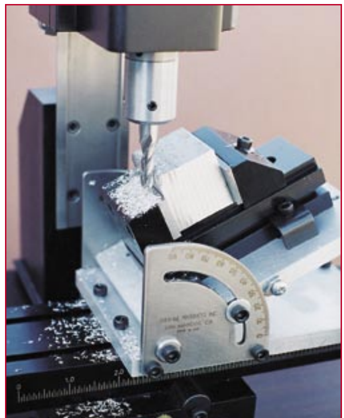
Figure 21—Chamfers can be milled using the tilting angle table on a mill.
