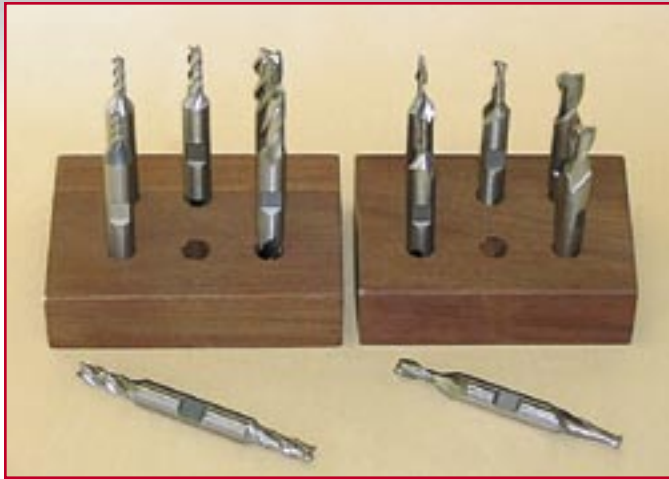
Figure 23—Double-ended 3/8" end mills fit in the P/N 3079 end mill holder. They are available in a large variety of sizes and shapes. For strength and maximum rigidity, use the largest diameter cutter your job will allow.
