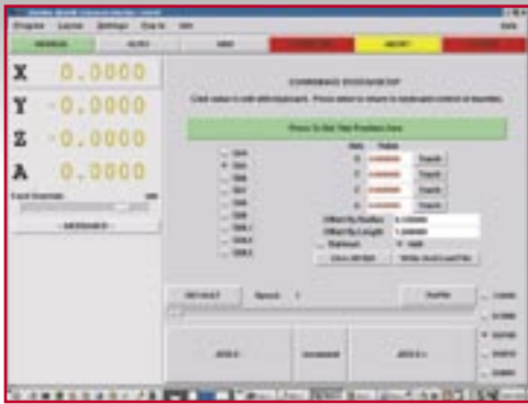
SAMPLE SCREENS: Coordinate systems offset screen also shows jog controls at bottom. (X-axis is highlighted)
