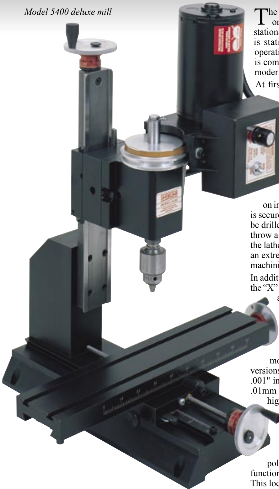
Figure 18—The saddle locking lever provides a positive lock for the Z-axis and is standard on all Sherline manual mills. CNC mills have a lock that also controls backlash.
