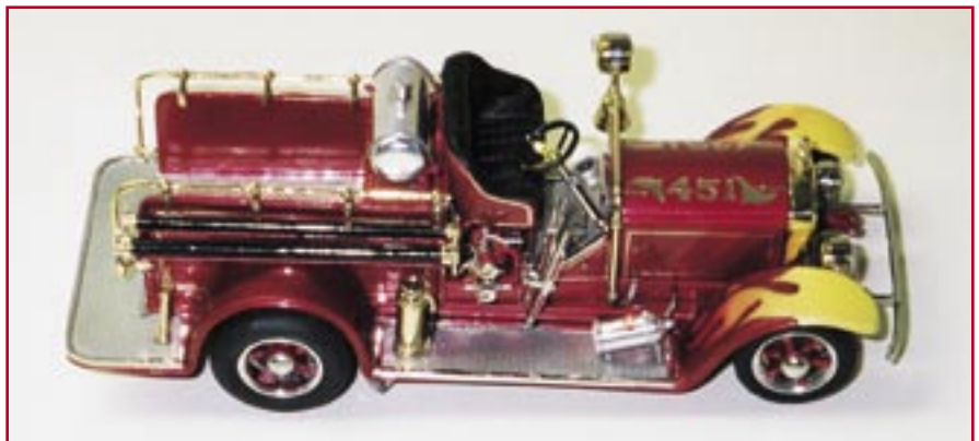
1/32 American LaFrance hotrod fire truck • Mike Foti, Hillsboro, OR Mike's entry in the hotrod division of the 1999 Salt Lake City national model contest is made entirely from formed and soldered brass. Items like the wheels, gas tank, lights, bell and rail stanchions are turned on the lathe.
