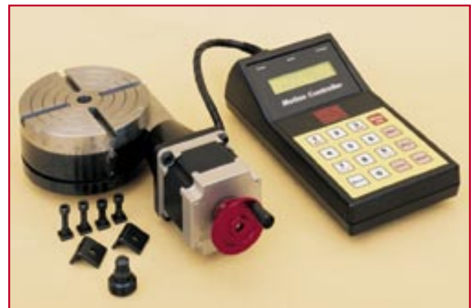
Figure 29—For complex indexing jobs Sherline's 4" rotary table is the perfect platform for the application of CNC controls. Included is a programmable input unit that contains its own microprocessor, keypad and power supply.
