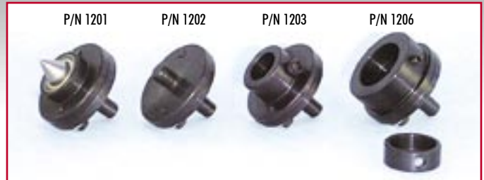
FIGURE 10—Adjustable tailstock tools make it possible to achieve "perfect" alignment between the headstock and the tool held in the tailstock. From left to right are the adjustable live center, adjustable drill chuck holder, adjustable custom tool holder and adjustable 1" die holder. The 1204 holder is similar to the 1202 but with a 0 Jacobs male taper to accept the 5/32" Jacobs chuck.
