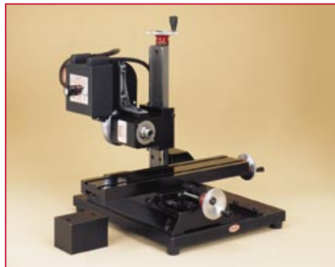
Figure 32—The horizontal milling conversion allows the mill column to be repositioned in two different ways on a sturdy base plate in order to provide greater versatility in set-up and increase the machinable area of the parts being worked on. To the left of the mill is the base of the Z-axis column, which has been cut off to allow a lower positioning of the headstock in relation to the table.
