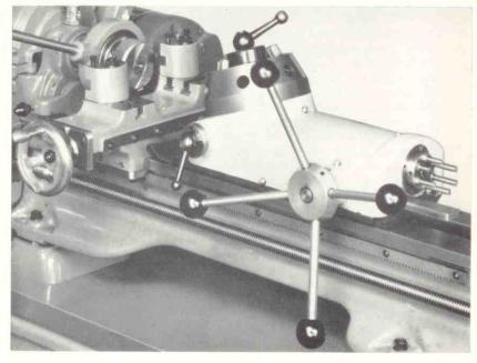
The illustrations show the turret slide, with and without tooling, mounted on an ML7BT Lathe. Also clearly visible are the 20/065 lever operated collet chuck and 1458 cut-off slide.
