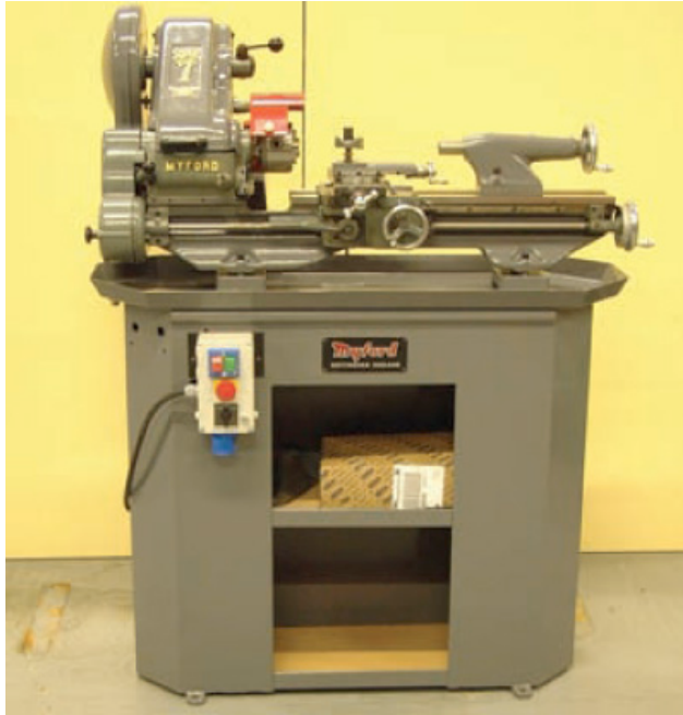
Photo 26 Back on its repainted cabinet stand, with new switchgear fitted, our reconditioned lathe awaits a new owner
