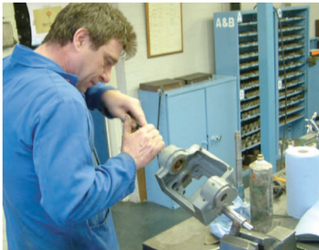
Photo 15 Brian McKechnie re-fits the front bronze taper bearing by scraping
