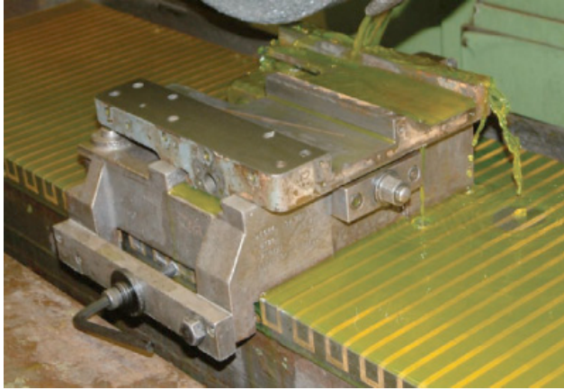
Photo 7 The saddle is mounted off the cross-slide dovetail to re-grind the under surfaces
