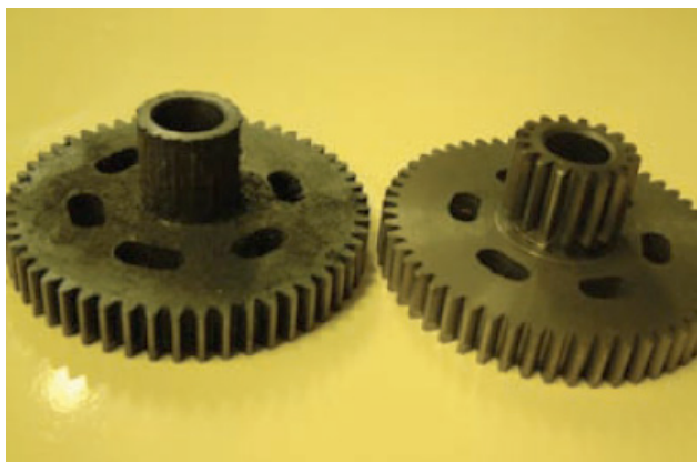
Photo 16 The old with the new. The back gear cluster had suffered badly, with no teeth left on the small pinion. The bull wheel was also short of its full complement, as can be seen in Photo 2
