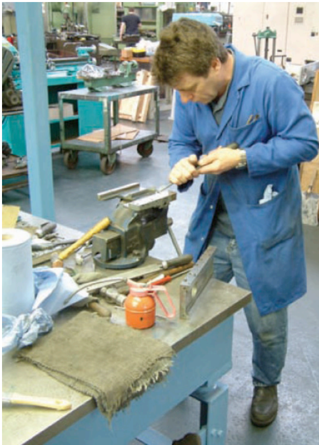
Photo 8 Brian McKechnie scrapes the underside of the saddle to produce a good bearing surface
