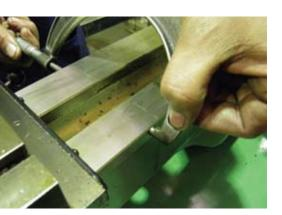
the thickness of the bedways (shears). A 1-2" (25-50mm) micrometer to check for wear across the front bed ways on narrow guide beds and a 4-5" (100-125mm) micrometer to measure across the bedways of a wide guide Series 7 Lathe bed. Finally a 5-6" (125-150mm) micrometer to measure across the bedways of a 254 Lathe.
