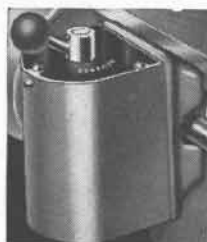
Fig. 24 Drum Type Switch Mounted on Switch Bracket
