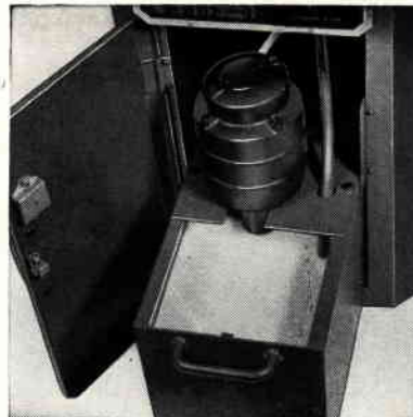
Lock-up Cabinet utilized for the internal mounting of Coolant Tank and Submersion pump.
