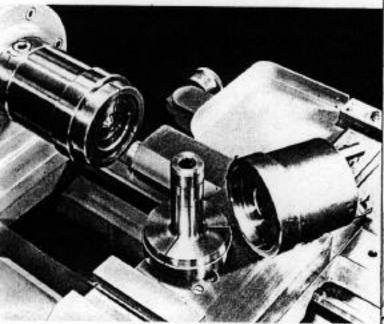
Available in 3", 4", 5" or 6" capacity • Attaches directly to cam lock spindle nose • Operated by either simple handwheel type drawbar (same as supplied with drawbar type collet attachment) or by lever operated pull type collet attachment.
