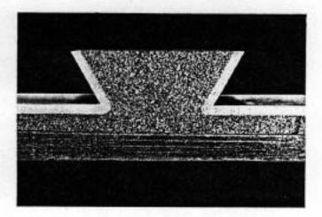
The dovetail of the carriage crossbridge is completely hardened to Scleroscope reading of 70 to 72 and ground.
