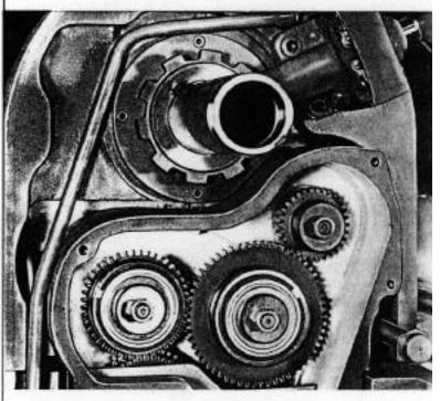
Totally enclosed and automatically lubricated • Gear train used only for thread chasing • Removal of cover permits quick change of gears for the securing of odd leads or the substitution of Metric transposing gears.
