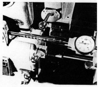
Precision type dial indicator, graduated in thousandths, mounted in bracket on left hand carriage wing • Stop bar with micrometer head carried by housing at front of headstock • Micrometer head in bed-mounted bracket also supplied for long work beyond lateral movement of regular stop bar.
