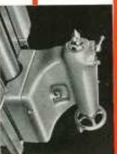
Tailstock incorporates correction device to ensure parallelism of work.
