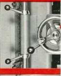
Travelling Traverse controls. Either hand operated or by automatic stops.
