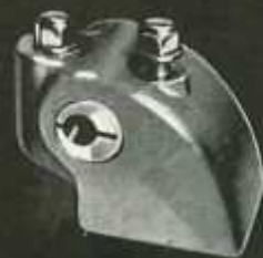
Internal Tool Block with eccentric Bush for accurate setting of the tool height.
