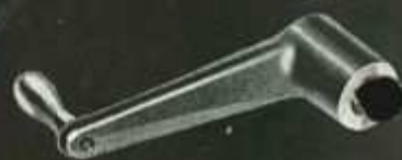
Lever for hand rotating the Lead Screw for setting up purposes.
