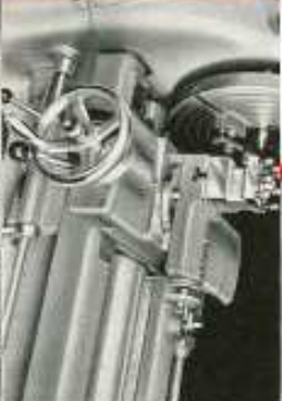
Strongly constructed Saddle. Protected Slideways. Large Micrometer Feed Dials and quick Tool Withdrawal Lever.
