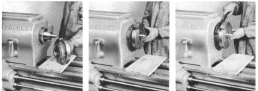
FIG. 57---MOUNTING FACE PLATES ON A REGAL IS QUICKLY ACCOMPLISHED THANKS TO THE TAPER KEY DRIVE SPINDLE NOSE WHICH HOLDS THEM SECURELY AT HIGH SPEEDS .
