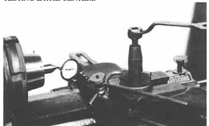
FIG. 82 - CHECKING FOR RUN-OUT
