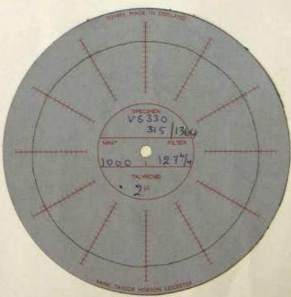
TALYROND graph indicates the deviation from true roundness on a sample workpiece turned on this lathe.
