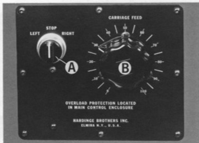
Figure 18—Power Feed Control Box
