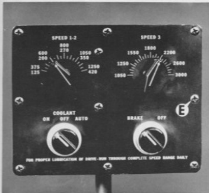
Figure 35 — Variable Speed Control Panel
