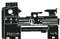
The tailstock is a large sturdy unit with a hardened precision sleeve and quick acting lock actuated by a lever. It has considerable projection so as to make it possible to work short pieces without excessive extension of the sleeve. It can be adjusted crosswise by turning slightly tapered gibbs. It is fitted with a graduated dial for measuring depth of cut.
