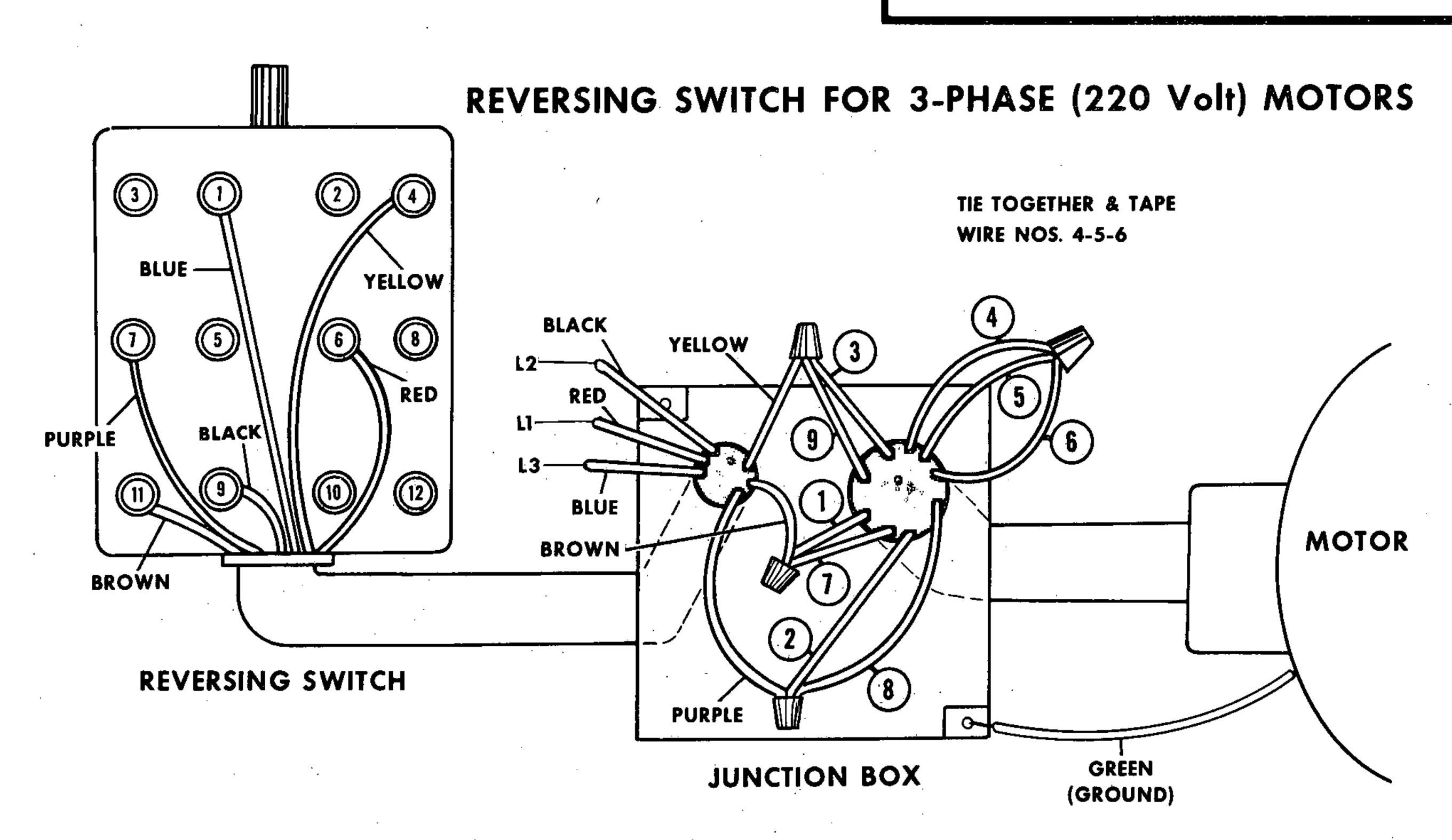
NOTE: TO REVERSE ROTATION OF MOTOR INTERCHANGE ANY TWO LINE LEADS L1, L2 OR L3.
