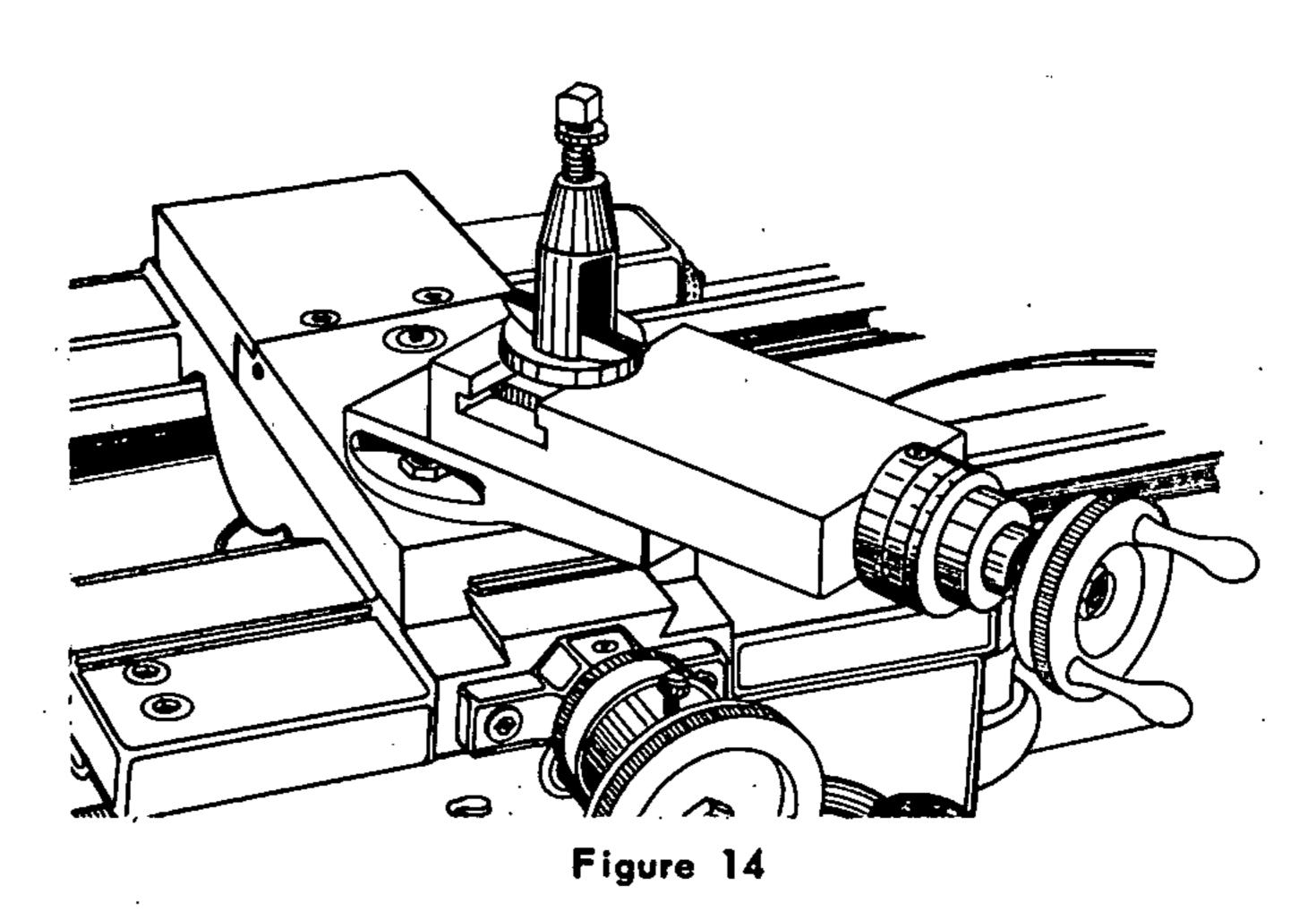
WRONG -- Tool post slide is too far back -- tool overhang is excessive -- refer to figure 14.
