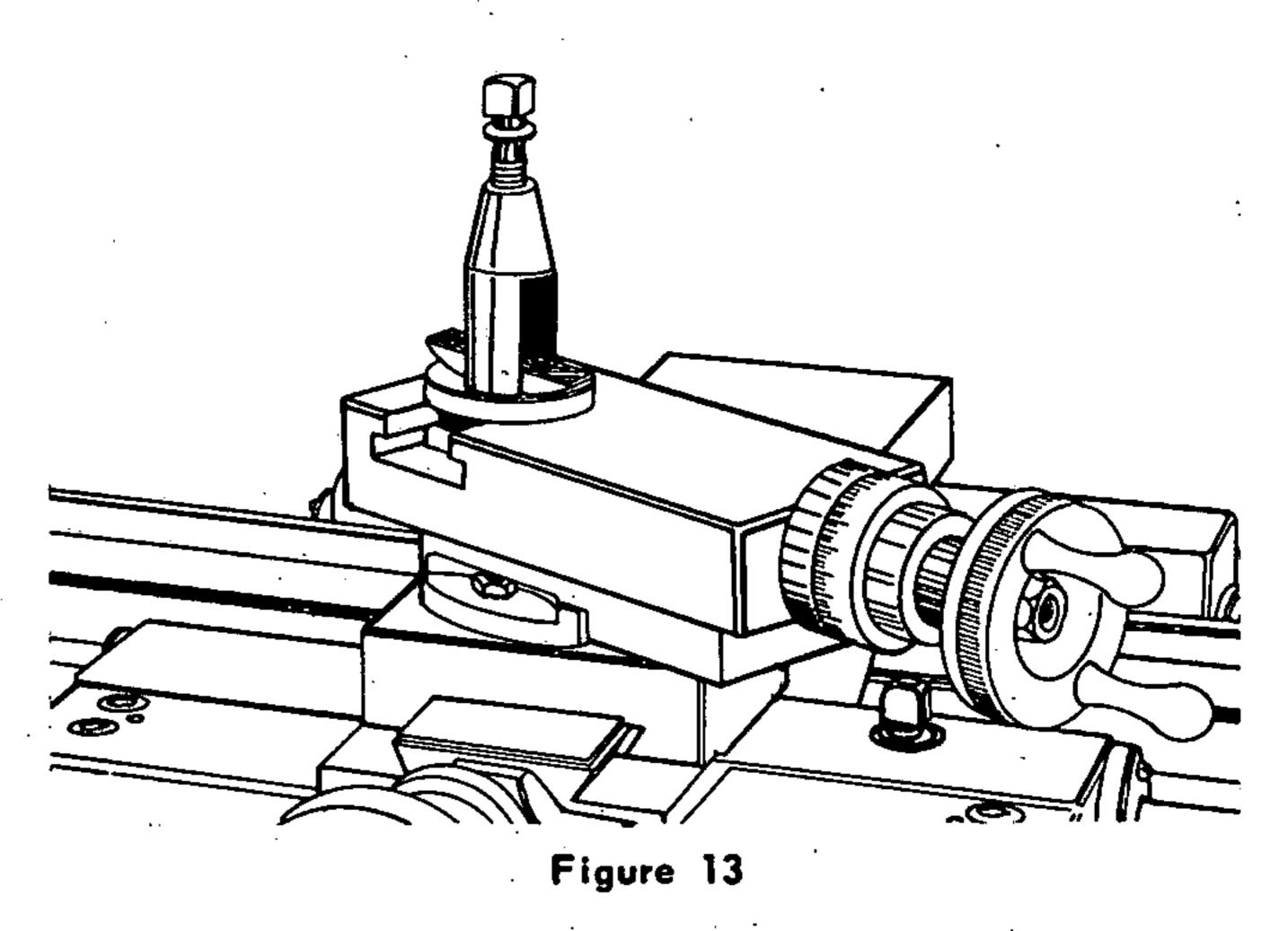
WRONG -- Unnecessary overhang of tool post slide will result in tool chatter, and could cause the tool post slide to break -- refer to figure 13.
