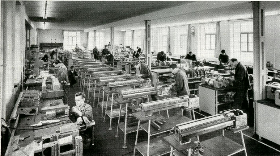
Assembly line Bed and carriage assembly Testing the reversing gear
