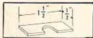
FIG. 2. Approximate shim dimension.
